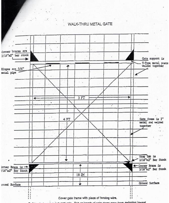
Build gate to swing outward only. Tab or length of gate stops gate from swinging inward.
